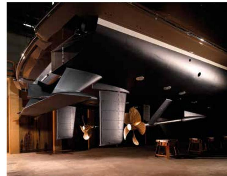
Heesen's motor yacht *Alive* is equipped with Van Oossanen's invention Hull Vane
