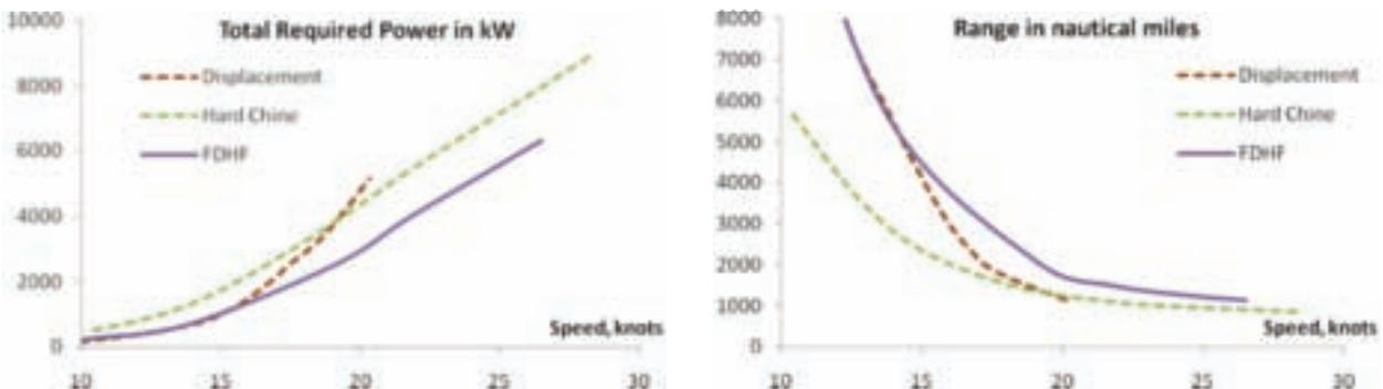
Figure 2. Power and range curves for the comparison
