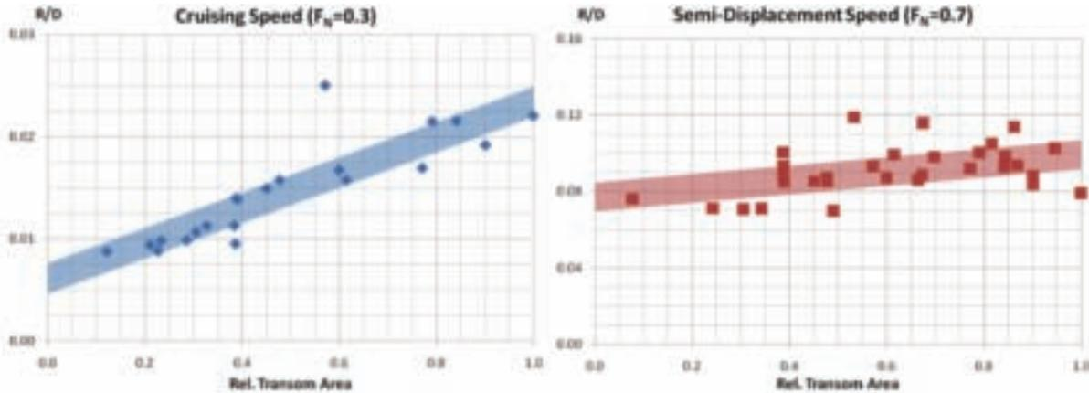
Figure 1. Dependency of resistance on the immersed transom area at  $FN_L = 0.35$  and  $0.60$ . The vertical scale displays the hydrodynamic resistance-per-ton of displacement and the horizontal axis shows the relative area of the transom below the water.
