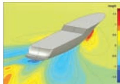
*Top image: 3D view of the computed wave elevations around the FDHF at semi-displacement speeds. The colours indicate the wave height, red being the highest value and blue the lowest.*
