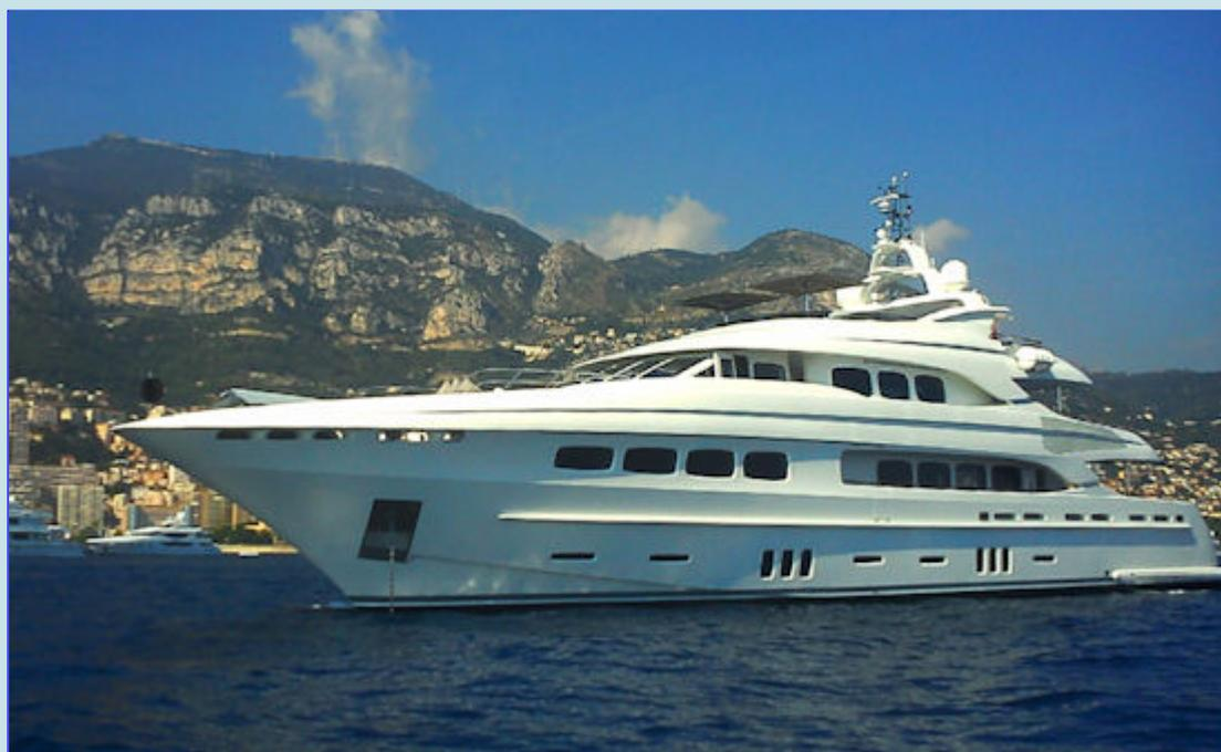
The superyacht sports a round-bilge semi-displacement hull designed by Van Oossanen & Associates. This allows for the combination of very economic sailing at displacement speeds between 10 and 15 knots, while her twin MTU 16V2000 M93 engines still have the juice (1790 kW each) to push the boat to 20.7 knots. There is no hump speed - the luxury yacht is equally at ease at all speeds in the range.
