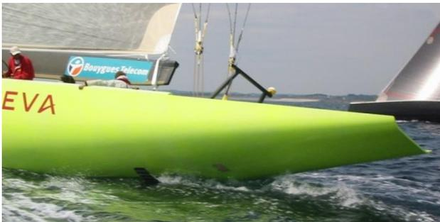
**Figure 1:** The second application of the Hull Vane<sup>®</sup>, on the 2003 IACC yacht *Le Defi Areva*.
