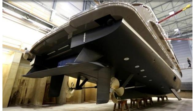
**Figure 2:** Application of the Hull Vane<sup>®</sup> on the 42 metre motor yacht *Alive*.
