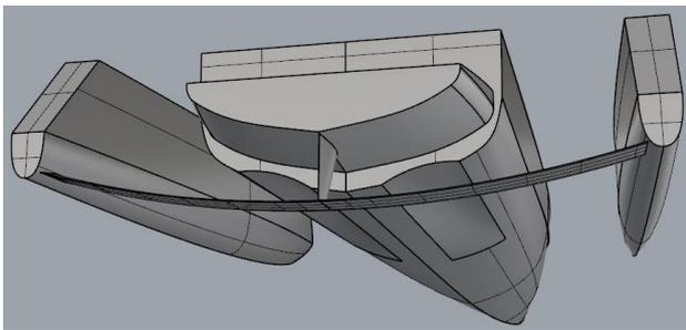
**Figure 6.** Perspective view of the trimaran configuration, including the Hull Vane<sup>®</sup>.
