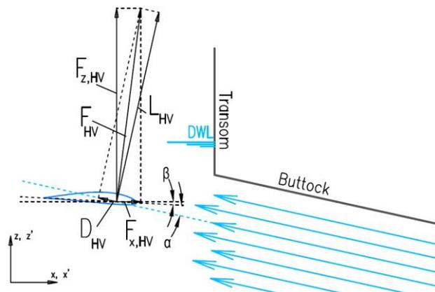
**Figure 3.** Schematic overview of the forces on the Hull Vane<sup>®</sup> in a section view of the aft ship. The vessel is displayed at zero trim.
