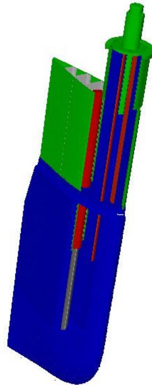
figure 2 Variable span rudder.
