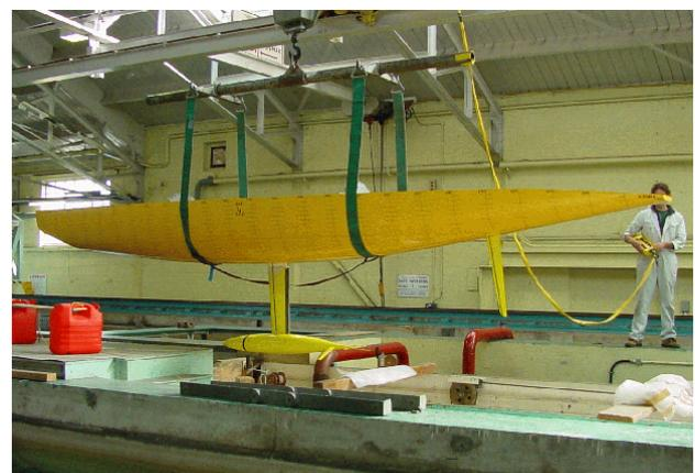
Figure 1: Tank testing model of a typical 2003 ACC yacht
