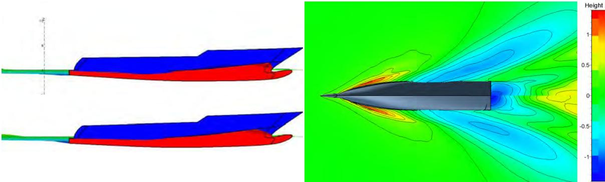
**Fig. 17.** Comparison of wave profiles (left) and wave elevations (right) for the Parent FDHF, with interceptor (top) and without interceptor deployed (bottom) at  $F_{NL} = 0.60$ .
