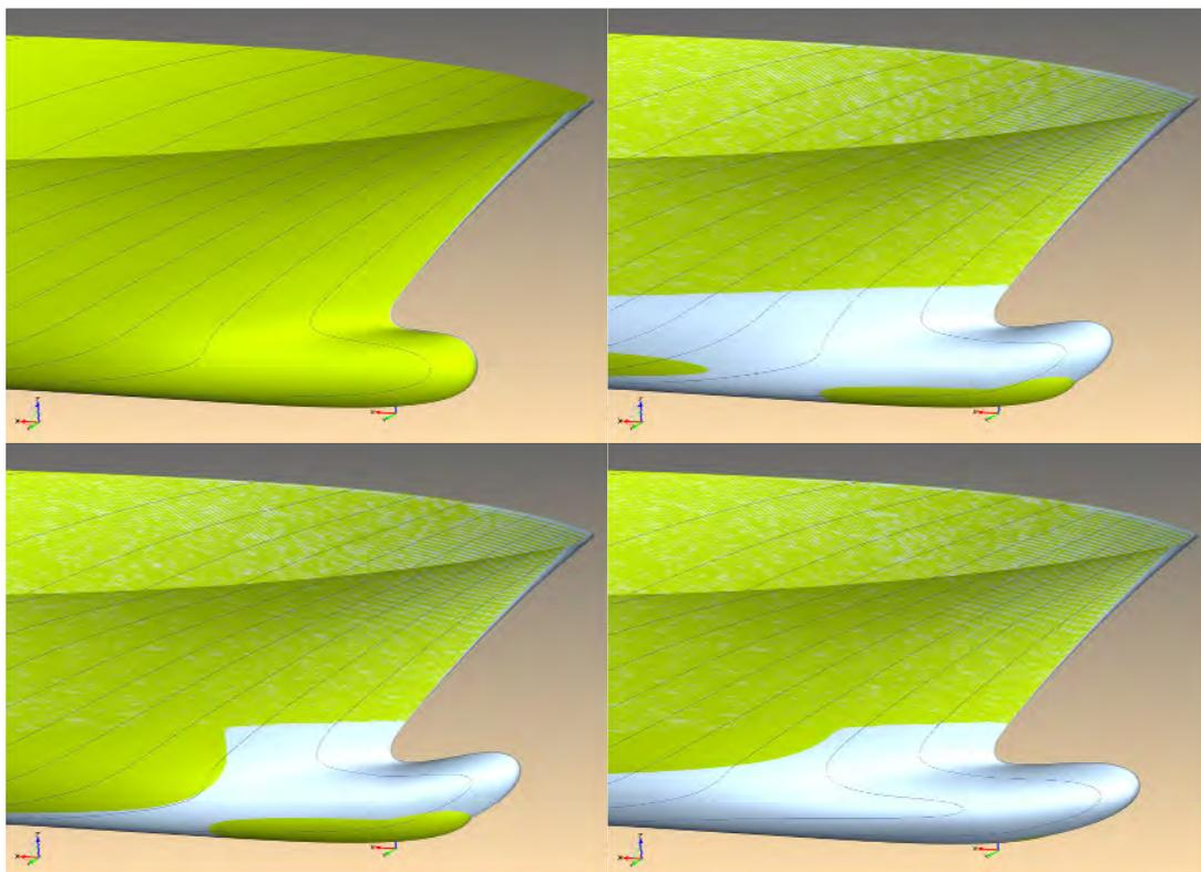
**Fig. 7.** Effect of variation of the deltaSurface parameters on the bow shape (light grey indicate varied surface regions); upper left: baseline hull to lower right: DoE favored design
