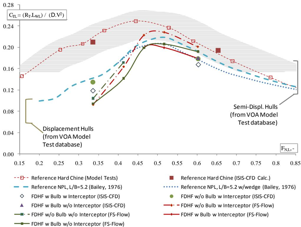
Fig. 14.  $C_{TL}$  values for the FDHF, reference Hard Chine and NPL Round Bilge Hull Form.
