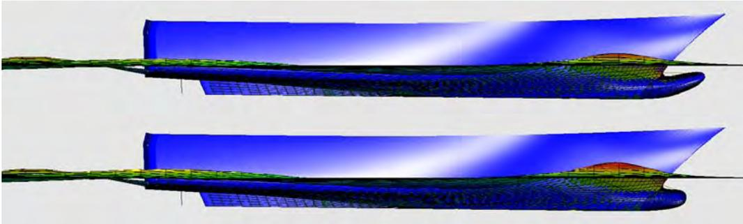
**Fig. 12.** Wave profiles along the optimized bulbous bow (top) and the bulbous bow before optimization (bottom)
