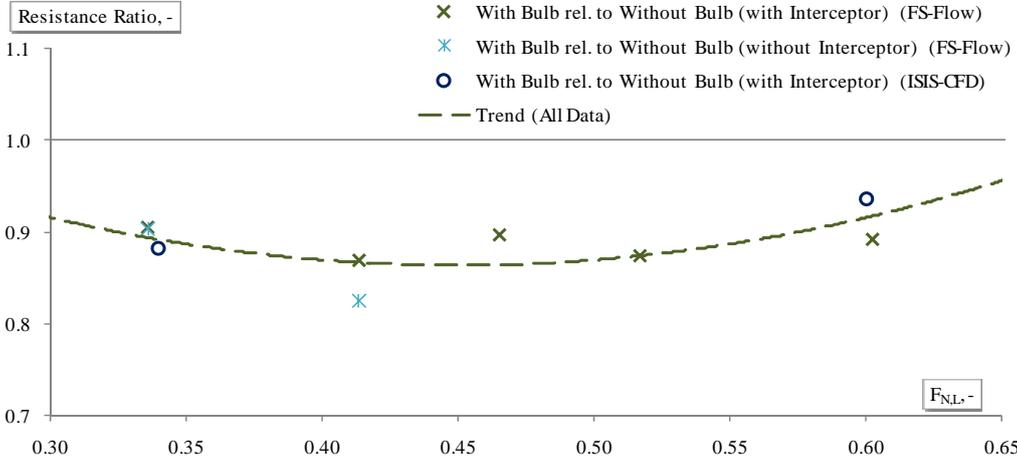
**Fig. 15.** Resistance ratio of the FDHF with bulbous bow, relative to the FDHF without bulbous bow, by using FS-Flow and ISIS-CFD.
