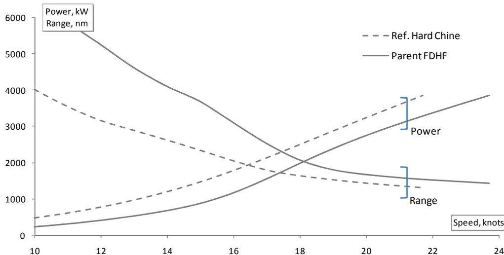
Fig. 18. Comparison of Power and Range for the FDHF and the reference hard Chine hull.
