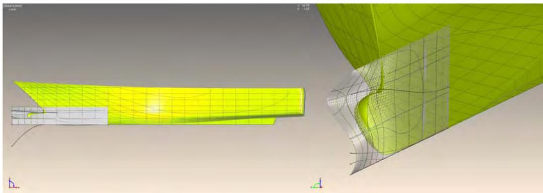
**Fig. 5.** Parameterized deltaSurface patch for variation of the bulbous-bow and entrance fairing region
