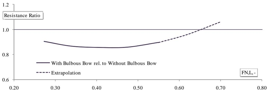
Fig. 3. Tank test results for a 44m motor yacht with and without bulbous bow.
