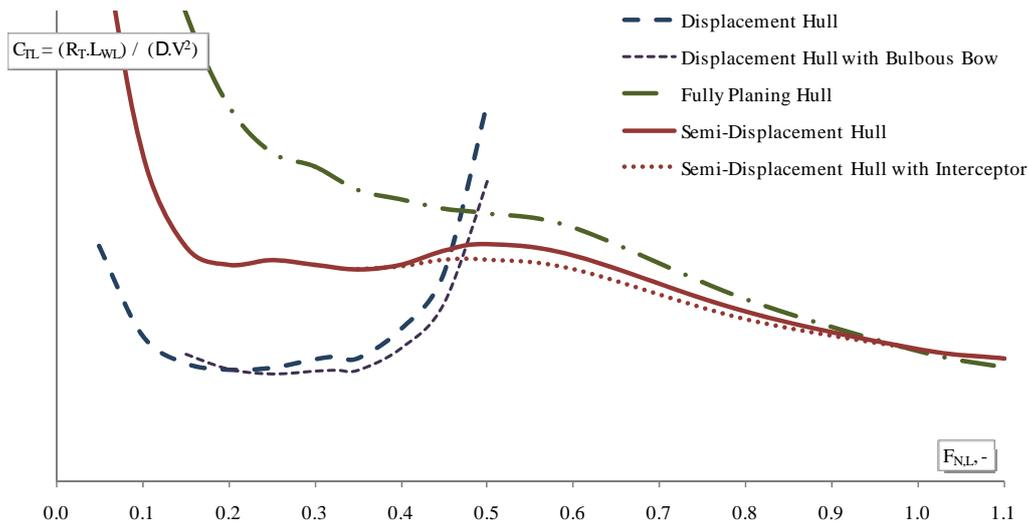
**Fig. 1.** Typical curves of  $C_{TL}$  for a displacement hull (with and without bulbous bow), a semi-displacement hard chine hull (with and without interceptor) and a fully planing hard chine hull.
