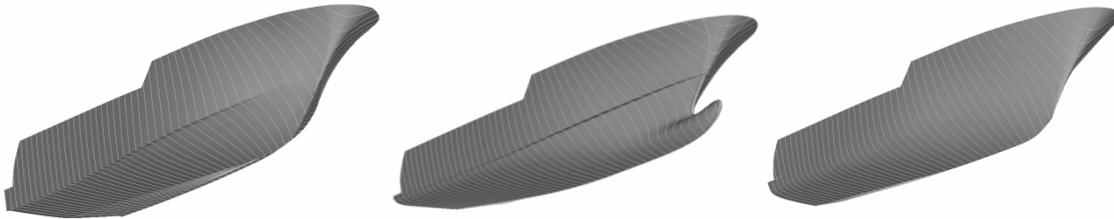
**Fig. 13.** Selected hull forms for the analysis: a hard-chine semi-displacement vessel (left), the equivalent Fast Displacement Hull Form with bulbous bow (middle) and the corresponding NPL Series Hull Form (right).
