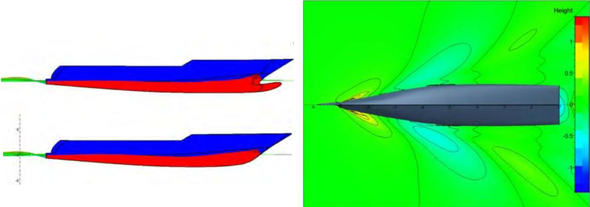
**Fig. 16.** Comparison of wave profiles (left) and wave elevations (right) for the Parent FDHF, with bulbous bow (top) and without bulbous bow (bottom) at  $F_{NL} = 0.34$ .
