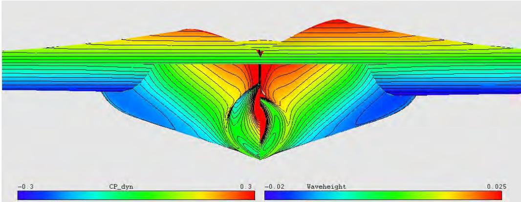
**Fig. 11.** CFD results for the bulbous bow optimization (dynamic pressure and wave height); left: optimized bulbous bow, right: bulbous bow before optimization
