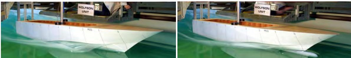
Fig. 4. Model at  $F_{N,L} = 0.55$  without bulbous bow (left) and with bulbous bow (right).
