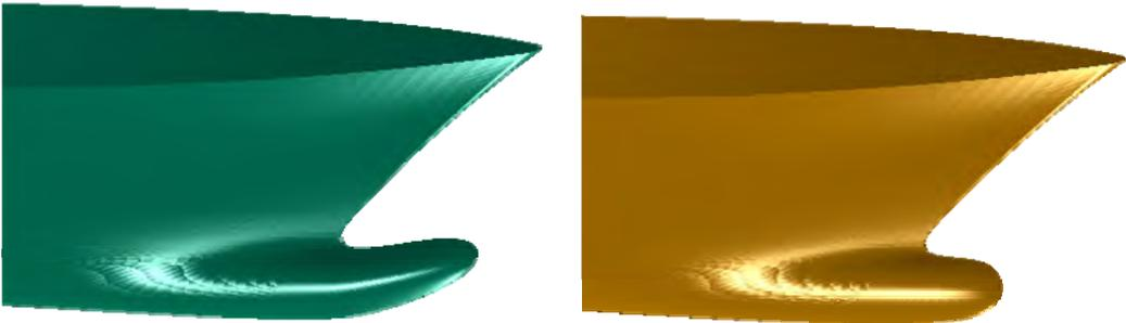
**Fig. 10.** Rendered views of the bulbous bow on a 47 metre motor yacht before (right) and after (left) a formal optimization
