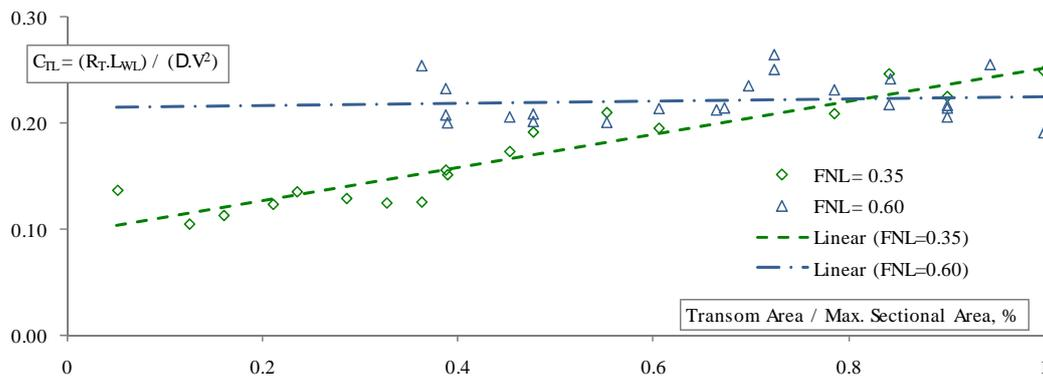
Fig. 2. Dependency of resistance (in the form of  $C_{TL}$ ) on the immersed transom area at a Froude number of 0.35.
