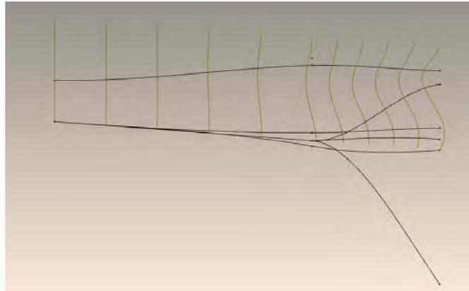
**Fig. 6.** Longitudinal curves defining the shape of the deltaSurface longitudinally and girthwise
