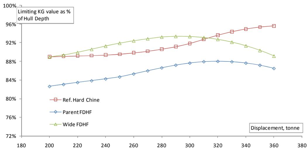
**Fig. 19.** Results of limiting KG analysis for the reference hard chine vessel and the parent FDHF, as well as for a widened FDHF model.
