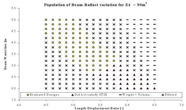
figure 5 Population of beam-ballast variation for a sail area of  $90 m^2$ .
