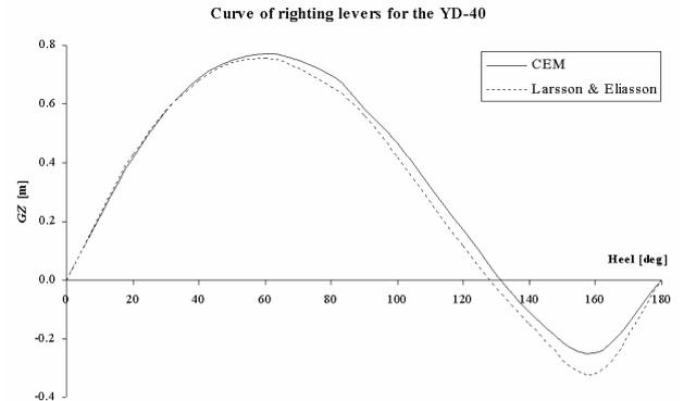
figure 3 Illustration of stability calculation results using Larsson and Eliasson's YD-40 [1].
